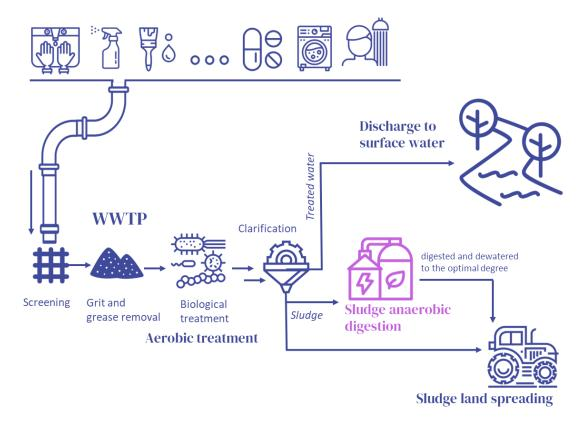
In WWTP, the larger fractions of water-insoluble chemicals, as well as of those which adsorb on to sewage solids, are bound to the primary settled sludge, which is separated from raw sewage in settlement tanks before the settled, or supernatant, sewage is treated aerobically. The sludge is then treated to heated digesters for anaerobic treatment.
